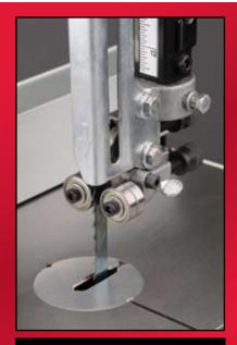
Upper and lower ball bearing guides reduce friction for longer blade life
